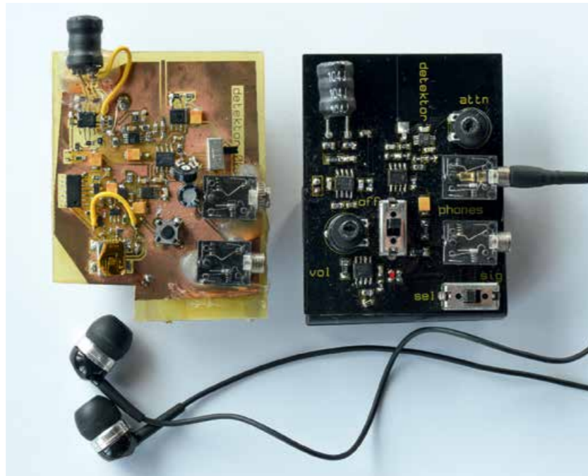
Detectors by Martin Howse and Shintaro Miyazaki – prototype and final PCB.
