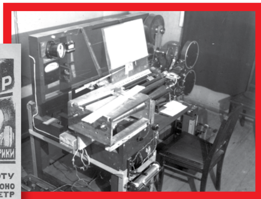
Evgeny Sholpo, Variophone, version two-three, late 1930s. Photo courtesy of Marina Sholpo.
